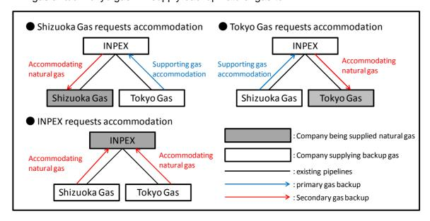
※ INPEX pipelines and Tokyo Gas pipelines are connected at Sano City, Tochigi Prefecture, Kawaguchi City and Kumagaya City, Saitama Prefecture. INPEX pipelines and Shizuoka Gas pipelines are connected at Gotemba City, Shizuoka Prefecture, where Minami Fuji pipeline of INPEX starts and ends.
