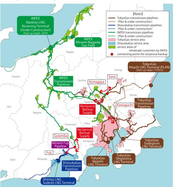
Premises of the backup supply of natural gas in an emergency The natural gas emergency backup scheme is based on the assumption that the three companies should secure their own stable natural gas sources. Backup gas volume and the terms etc under the Agreement will be decided and agreed after the negotiations by the three companies when natural disasters occur.
